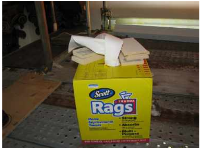
The cleaning method was a light spray of distilled water on clean Scott industrial towels. The towels are non-woven highly absorbent shop towels.
